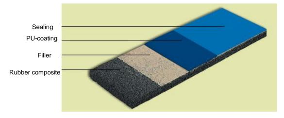
Outdoor: rubber composites are used as shock pads for artificial turf
